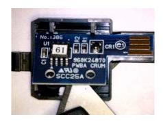
The board can now be lifted up and away from the last two retaining clips leaving the empty holder
