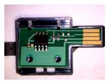
Reverse the procedure to install the new chip. Place the board edge under the two retaining clips on the holder.
