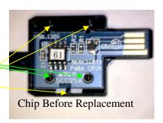
Using a hobby knife or similar place the blade under the pillar side of the board and GENTLY lever the board away from the fixing clip on that side
